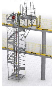
> 4 - Install the side gangway on the Escalib Mills. Assemble the braces on the 2<sup>nd</sup> MDS Gangway Bracket with M12-100-8.8 bolts. Install the anti-lifting device and of the gangway. Unsling.
