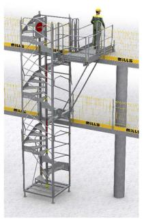
> 5 - If necessary, install the front gangway on the side gangway and bolt with M12-100-8.8. Open the guardrails for the passage.
