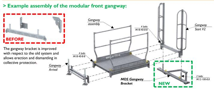
The MDS Gangway Bracket can be assembled with the front & the side gangways. We recommend delivering the gangway entirely assembled, ready to be lifted.
