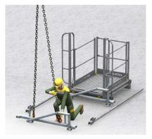
> I - Erect the side gangway prior on the ground, with the Start and an MDS Gangway Bracket. Sling the 2<sup>nd</sup> MDS gangway bracket.
