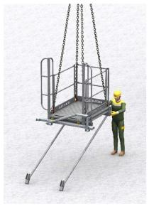
> 3 – Sling the side gangway. Install the braces at breast height with M14-100-8.8 bolts.
