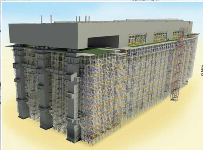
A BIM approach was applied for studying and assembling the Touréchaf falsework equipped with Mills Escalib access for the GTA table of the future Hinkley Point EPR power plant in England.
