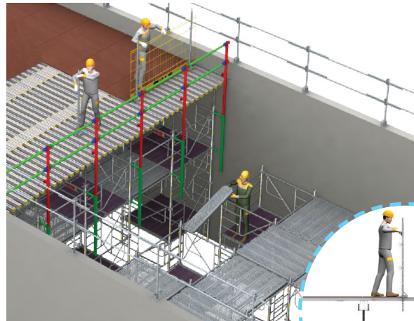
> 2 - Lay the plywood and temporary mesh barriers thanks to post universal supports. Assemble the second part of the falsework.
