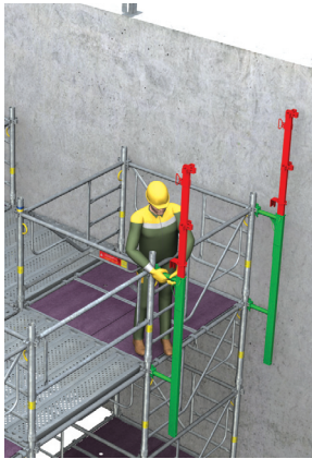
> 1 - Install two GCC uprights from the falsework decking.
