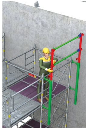
> 2 - Install two GCC ledgers on the uprights.
