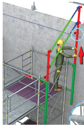
> 3 - Extend the first GCC upright so that the visual indicator is levelled with the future formwork. Lock the upright with the captive pin.
